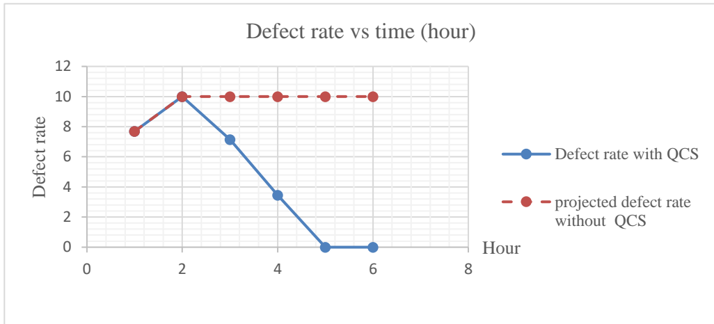
Figure 11: The 4's defect rate with QCS against projected defect rate without QCS
